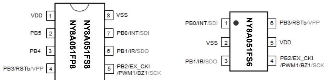
Figure 1 Package pin assignment
