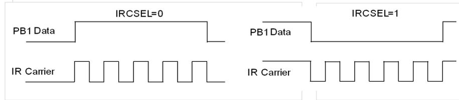
Figure 15 Polarity of IR Carrier vs. Output Data
