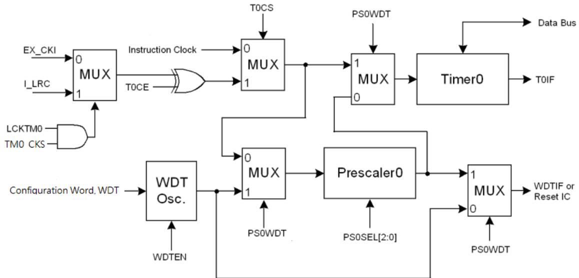
Figure 10 Block Diagram of Timer0 and WDT
