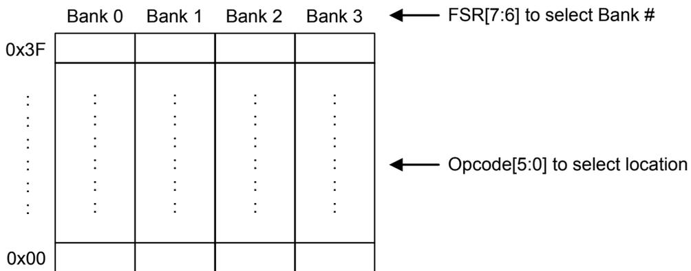
Figure 4 Direct Addressing Mode of Data Memory Access
