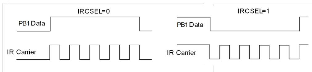
Figure 27 Polarity of IR Carrier vs. Output Data
