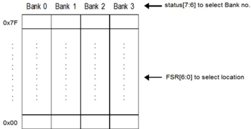
Figure 3 Indirect Addressing Mode of Data Memory Access
