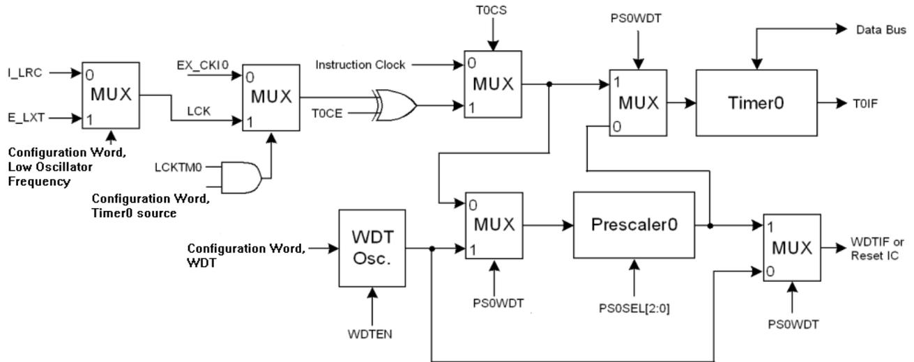
Figure 15 Block Diagram of Timer0 and WDT
