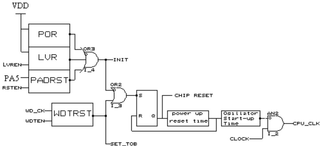
Figure 34 Block diagram of on-chip reset circuit
