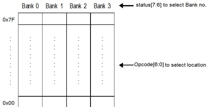
Figure 4 Direct Addressing Mode of Data Memory Access
