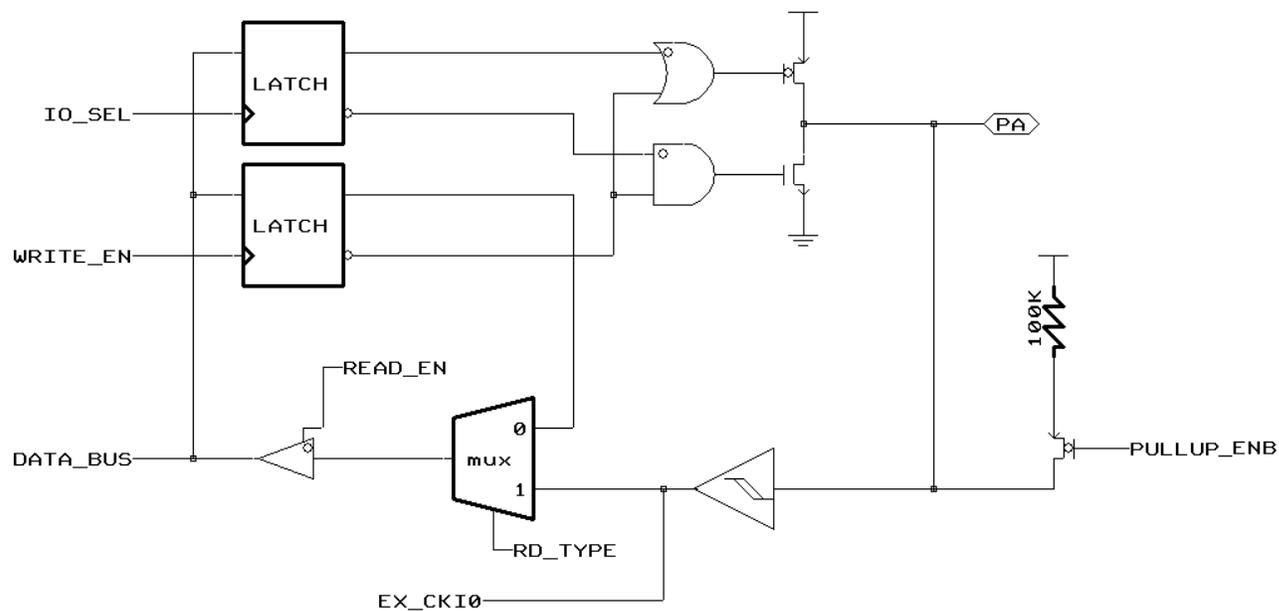
Figure 7 Block Diagram of PA4
